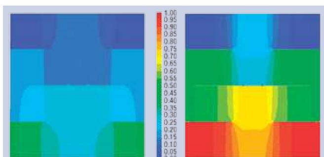
**FIG. 11** Pressure distribution through the shell for poor (left) and optimal (right) design.
