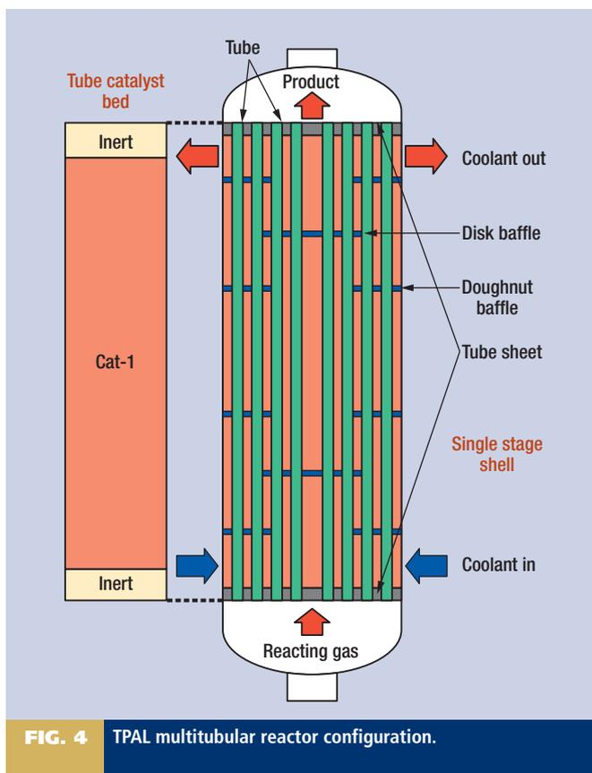
FIG. 4 TPAL multitubular reactor configuration.
