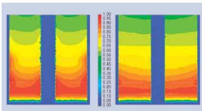
**FIG. 14** Tube center temperature distribution through the shell for poor (left) and optimal (right) design.
