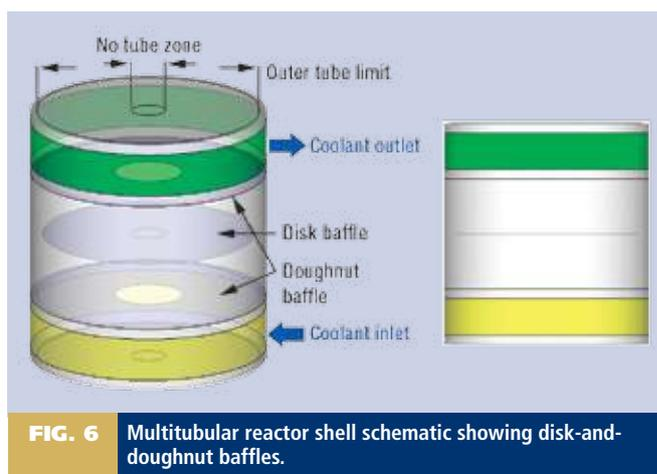
FIG. 6 Multitubular reactor shell schematic showing disk-and-doughnut baffles.
