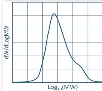
Detailed kinetic modelling considers elementary polymerisation reaction steps in chemically-initiated free radical polymerisation. The model solves for the evolution of the full molecular weight distribution (MWD) using the fixed pivot technique.
