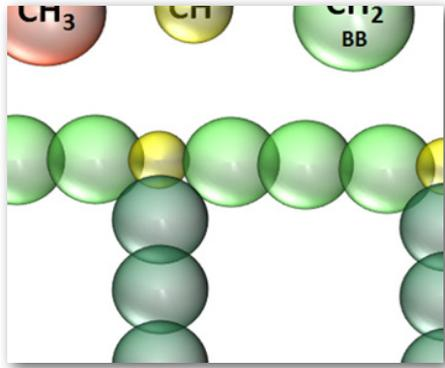
The Statistical Association Fluid Theory (SAFT)  $\gamma$ -Mie Equation of State represents molecules as chains of distinct functional groups. Branching is accurately modelled, to provide accurate polymer properties across the MWD. This approach is ideally suitable for the modelling of polymers.
