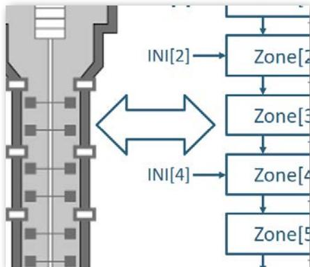
The hybrid multizonal approach couples a "cold-flow" Computational Fluid Dynamics (CFD) simulation of the reactor with the full chemistry model to represent both the polymerisation process and the complex flow pattern in industrial-size autoclave reactors.
